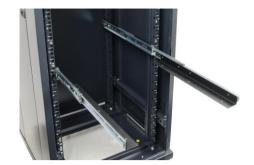
**3.2.** Place the ARAD enclosure onto the slid-out ARAS rails. Next, bolt it from the inside with 6xM4 screws (included). The enclosure is to be fixed to the front part of the RACK rails with four M6 screws.
