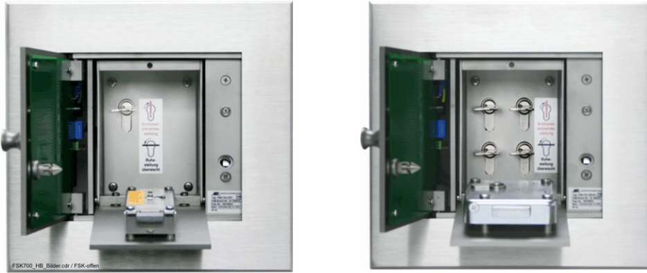
Fig. 2: Series FSK700 Fire Brigade Key Safe On the left: FSK700-2 with open outer and inner doors, master key inserted, inner door fitted with a double-bit variable lock On the right: FSK700-2SX with 4 master keys, open outer and inner doors, inner door fitted with a lock for a locking half cylinder
