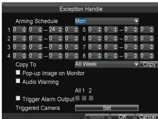
Figure 3.5 Linkage Actions of Motion Detection
