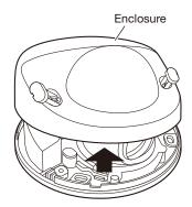
Detach the dome cover from the enclosure by removing the fixing screws. (Refer to the illustration described beside step 5.)
