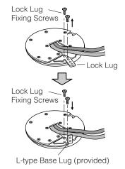
**7** Remove the two Lock Lug Fixing Screws and replace the Lock Lug with L-type.
